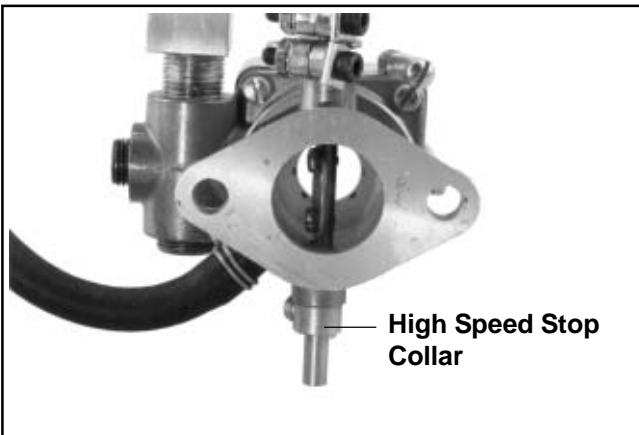
Figure 5A-11. Full Throttle Position.
